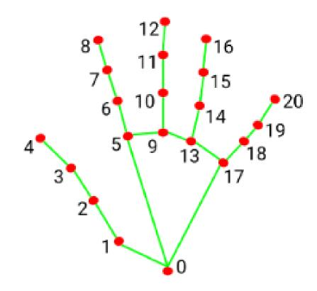
0. WRIST 11. MIDDLE\_FINGER\_DIP 1. THUMB\_CMC 12. MIDDLE\_FINGER\_TIP 2. THUMB\_MCP 13. RING\_FINGER\_MCP 3. THUMB\_IP 14. RING\_FINGER\_PIP 4. THUMB\_TIP 15. RING\_FINGER\_DIP INDEX\_FINGER\_MCP 16. RING\_FINGER\_TIP 6. INDEX\_FINGER\_PIP 17. PINKY\_MCP 7. INDEX\_FINGER\_DIP 18. PINKY\_PIP 19. PINKY\_DIP 8. INDEX\_FINGER\_TIP 9. MIDDLE\_FINGER\_MCP 20. PINKY\_TIP 10. MIDDLE\_FINGER\_PIP
